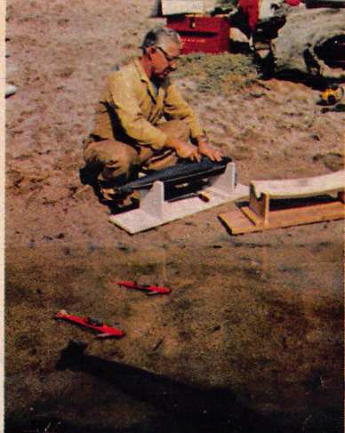
Above: Technician Wesley Lee prepares 31-inch sub for water. Below: Part of the fleet. The submarines were designed by Irwin Allen, creator and executive producer of Voyage, and by the Fox art department. They were first sculptured in wood and plaster, then they were cast in fiberglass.
